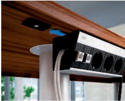
Mounting of the Deskbox on the fastening set, under-table mounting The Deskbox can be slid onto the fastening elements from the side. The design panel must be removed in advance.
